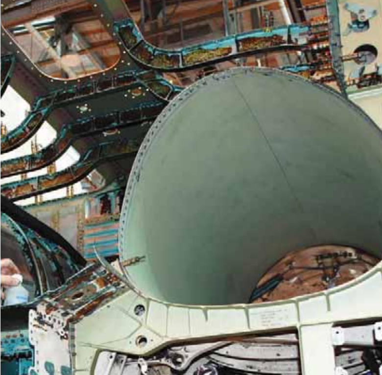
Joseph Stevens, a sheet metal mechanic at Fleet Readiness Center Jacksonville, Fla., prepares to install a center barrel on an F-18 Hornet. Managed by the Defense Supply Center Richmond, Va., Defense Logistics Agency Jacksonville supports FRC mechanics with spare and repair parts.
